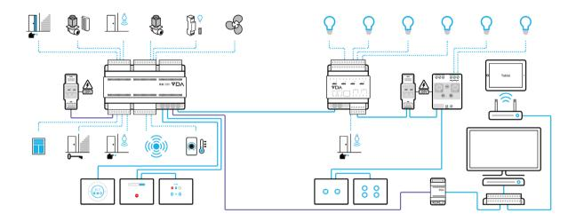
Our Micromaster system can be expanded and integrated with a wide catalogue of expansions and gateways to achieve any kind of integration with HVAC manufacturer, Lighting protocol or door lock systems.
